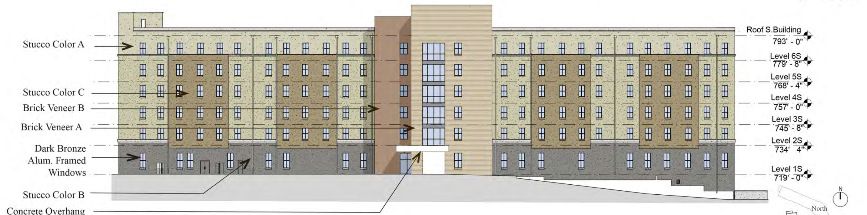
South Building - Southwest Elevation A2.00 1/32" = 1'-0" 0' 8'-0" 16'-0" 32'-0" 64'-0"
